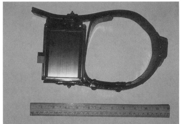
Fig. 1. Global Positioning System (GPS) radiocollar tested on wolves and white-tailed deer. Molded plastic box is 8.2 x 11.9 x 5.4 cm; the entire collar weighs 920 g.
